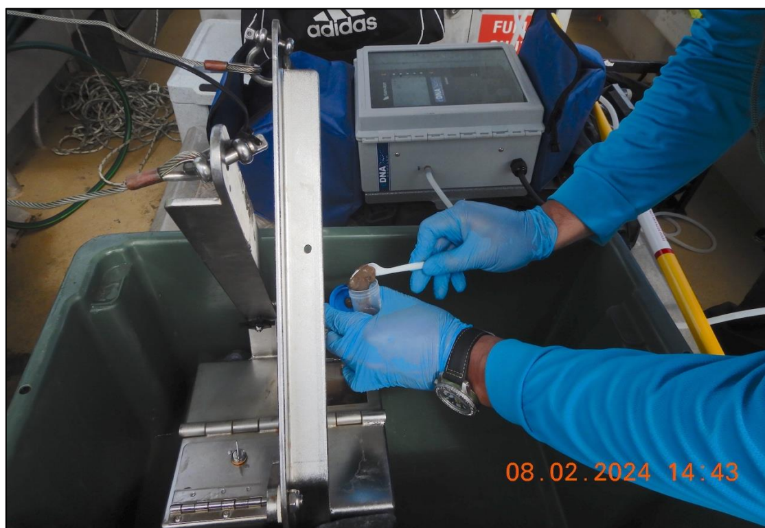
Figure 4. Taking sediment samples from the grab.
