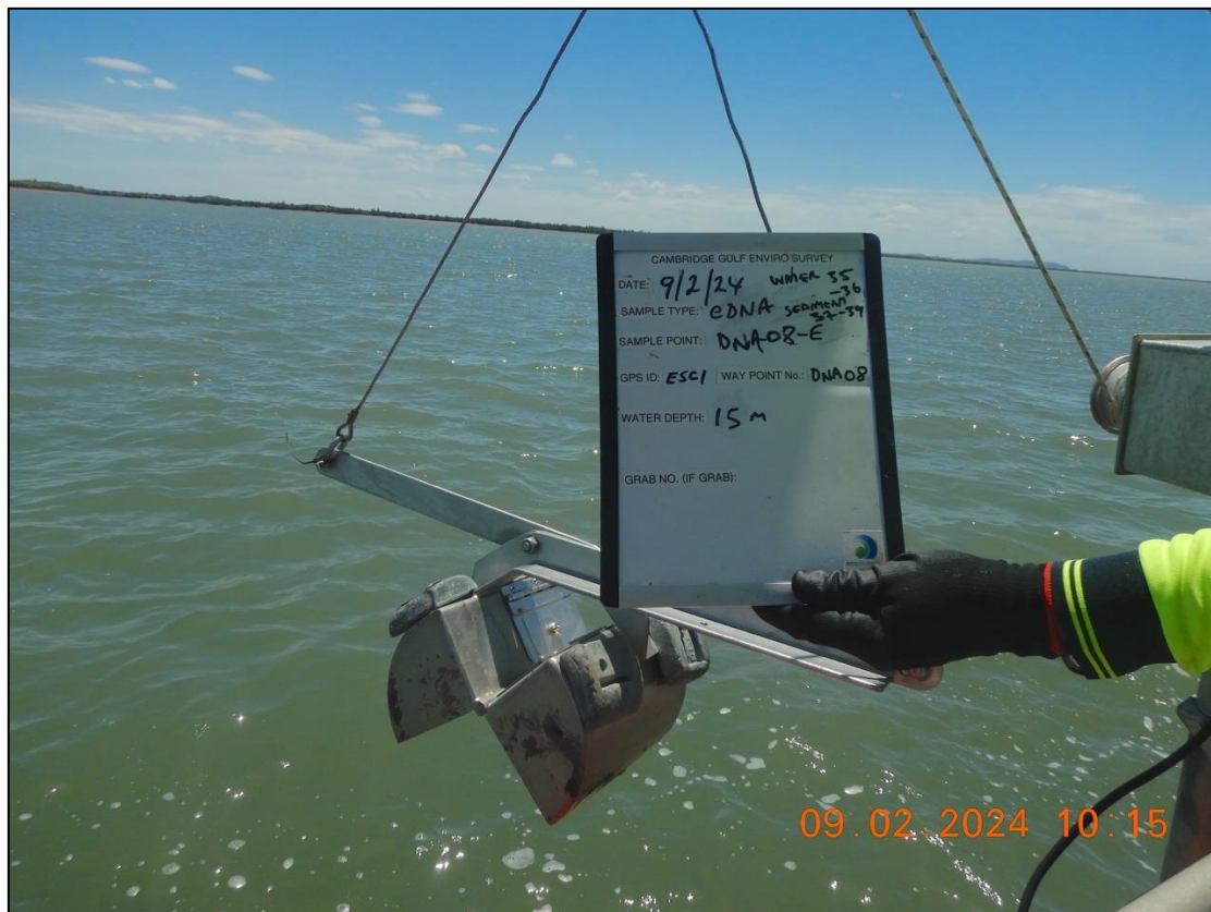
Figure 3. Grab used for taking seabed sediment samples.
