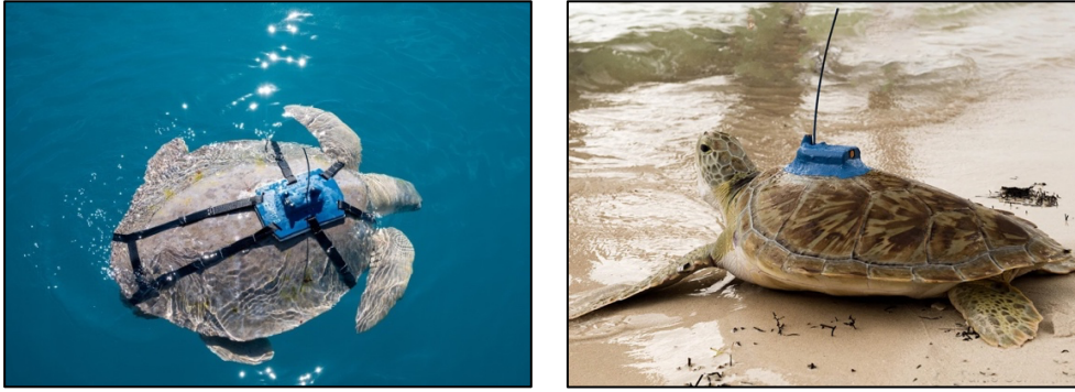
FIGURE 1: Examples of satellite trackers attached to marine turtles - attached by straps (left) or epoxy glue (right).
