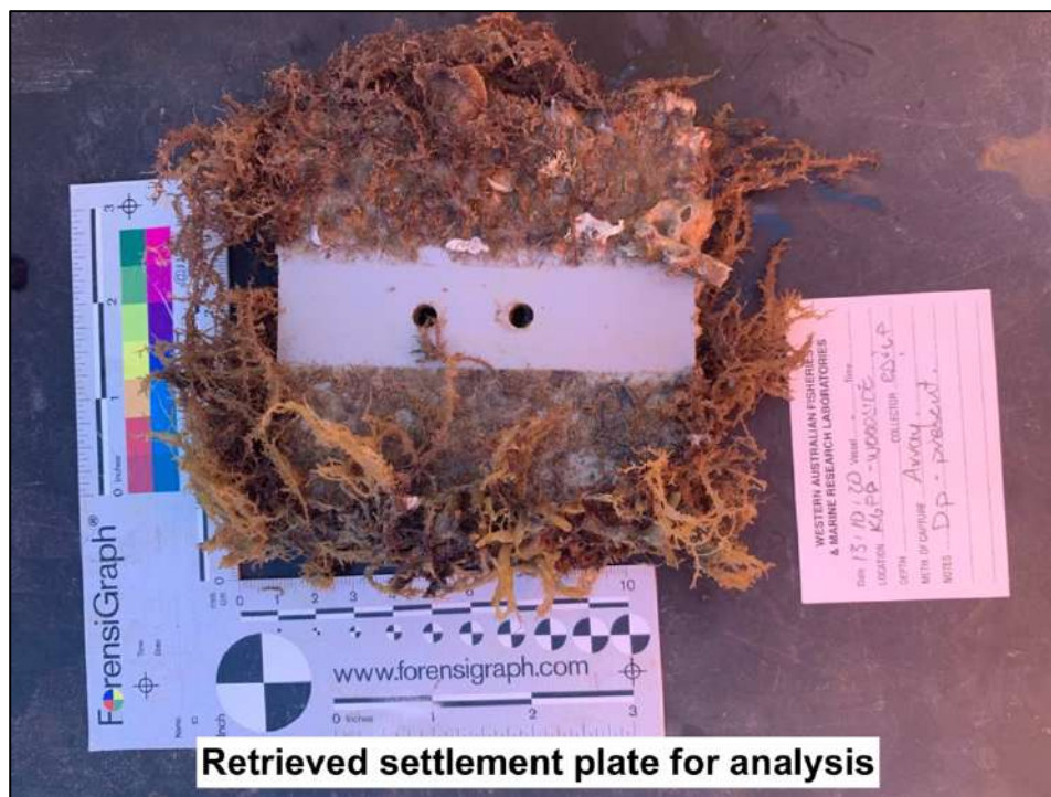
FIGURE A1.3: SWASP settlement plate after deployment, ready for analysis (source: DPIRD)
