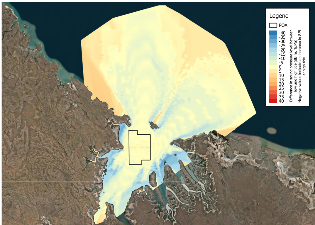
Figure 10 Difference in the radiated sound pressure level between a 3.25 m high tide and a -4 m low tide in an east-west transect.
