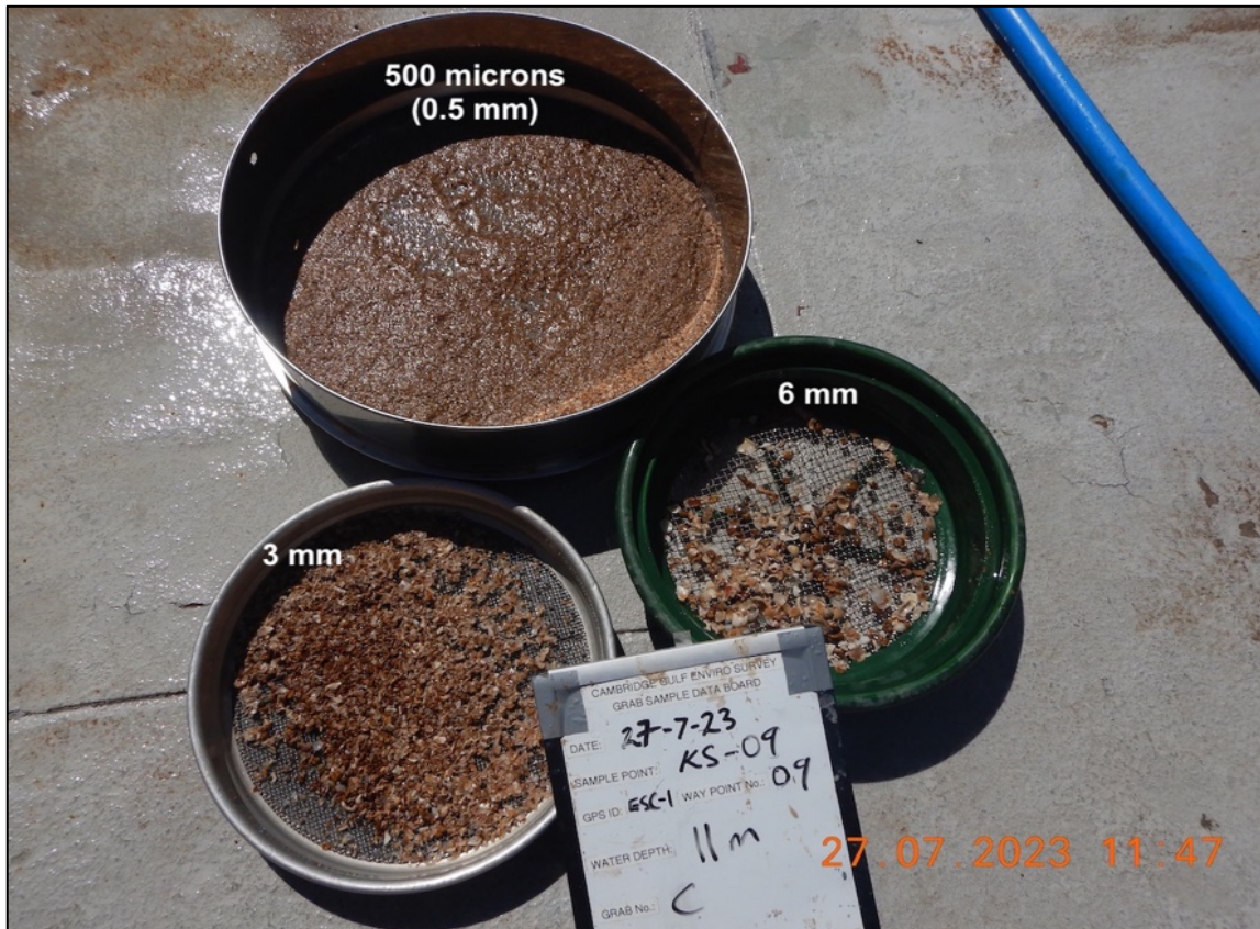
FIGURE 6.28: In some samples the sediment type, especially samples where the grab returned a full five-liters of sand, required pre-sieving using a 3 mm or even 6 mm sieve, followed by the 500-micron sieve.
