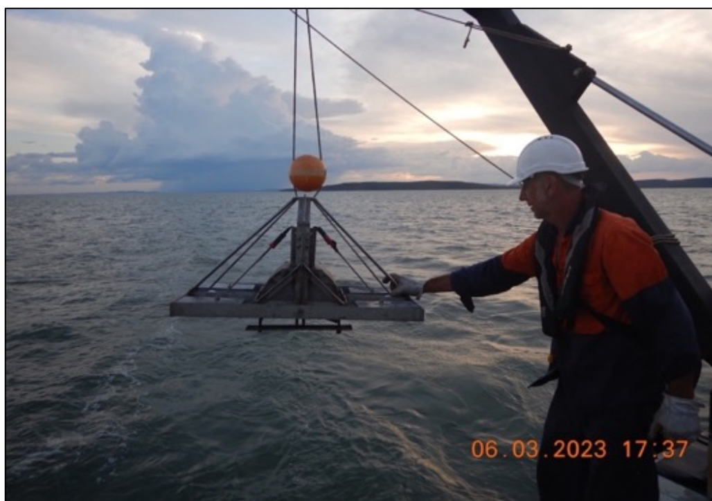
FIGURE 6.20: The five-litre Smith-McIntyre grab used for the benthic sampling in CG.
