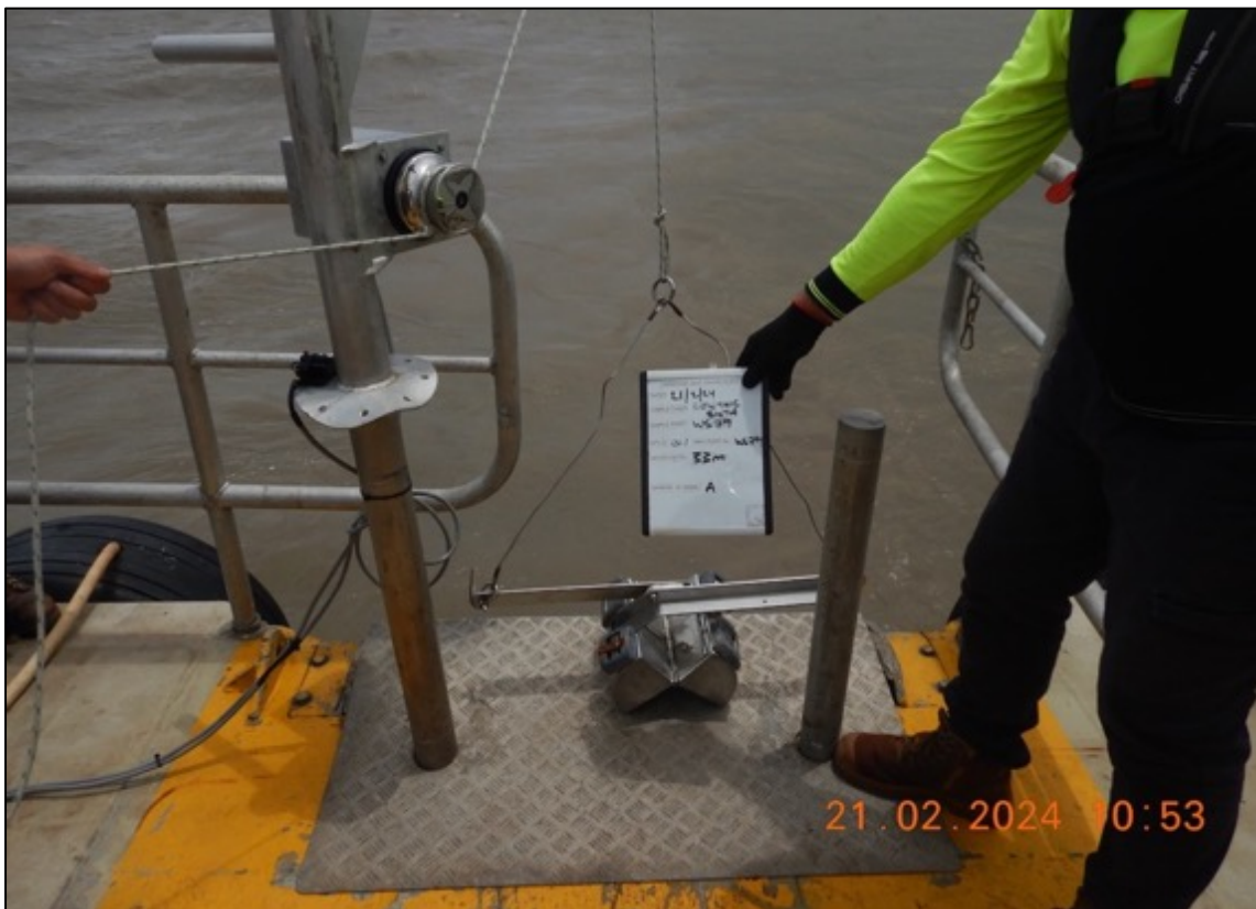
FIGURE 6.24: A data board was photographed with the grab before each deployment, to provide a complete date-time stamped photographic record of all steps in each grab cycle.
