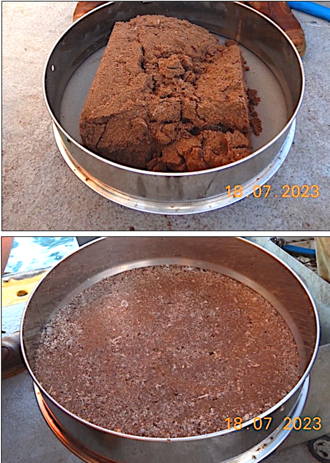
FIGURE 6.40: An example of a grab sample of sand from within the POA. Top is pre-sieve and bottom is post-sieving to 500 microns, which was then searched for biota. Most sand samples did not contain biota, as constant movement of the sand under tidal currents prevents colonization. Compare this with Figure 6.42.
