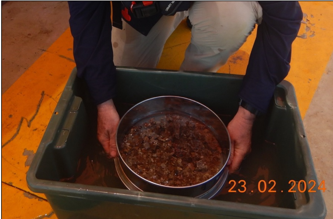
FIGURE 6.30: For courser sediments like shell-grit and gravel, after initial sieving and biota assessment, the sieve and retained sediment was returned to a bin of seawater with the water ~1 cm above the sediment surface, then gently shaken. This 'floated off' any small organisms that might have been missed visually amongst the sieved sediment.
