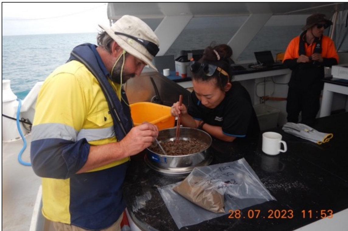
FIGURE 6.29: Post-sieved material was sorted and inspected in detail in-situ in the sieve, using chop-sticks and forceps to remove any biota found, as well as pipettes for very small biota. Samples were assessed by two people.
