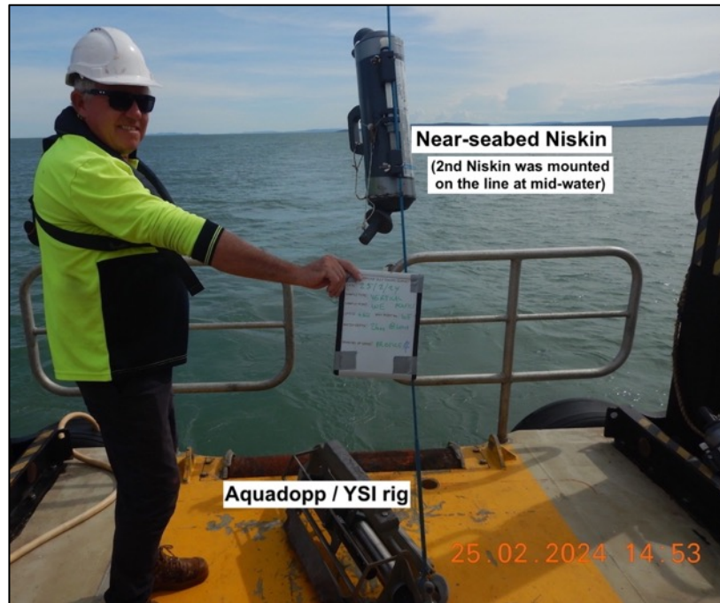
FIGURE 8.9: Equipment set-up for Vertical Water Quality Profile sites in CG wet season Feb 2024, with near-seabed Niskin shown. A second Niskin was fitted to the line at the mid-water point as the rig was lowered to the seabed.
