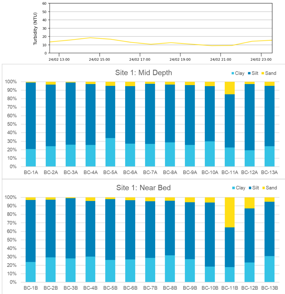
Figure 113. Measured near-bed turbidity (top) and composition of the suspended sediment at mid depth (middle) and near-bed (bottom) over a spring tidal cycle at Site 1. Note: the high percentage of sand sized particles in samples BC-11A, BC-11B and BC-12B are due to sand sized organic matter being present, the actual percentage of sand will have been in line with the other samples (i.e. around 5%).
