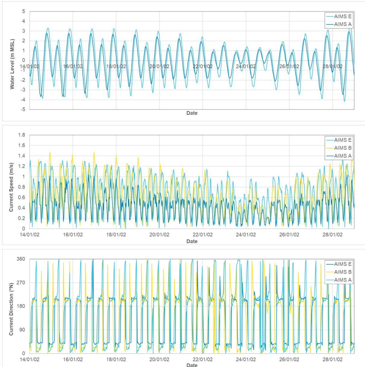
Figure 21. Measured water level and current speed and direction at mid-depth at AIMS A, B and E (source: AIMS, 2007).
