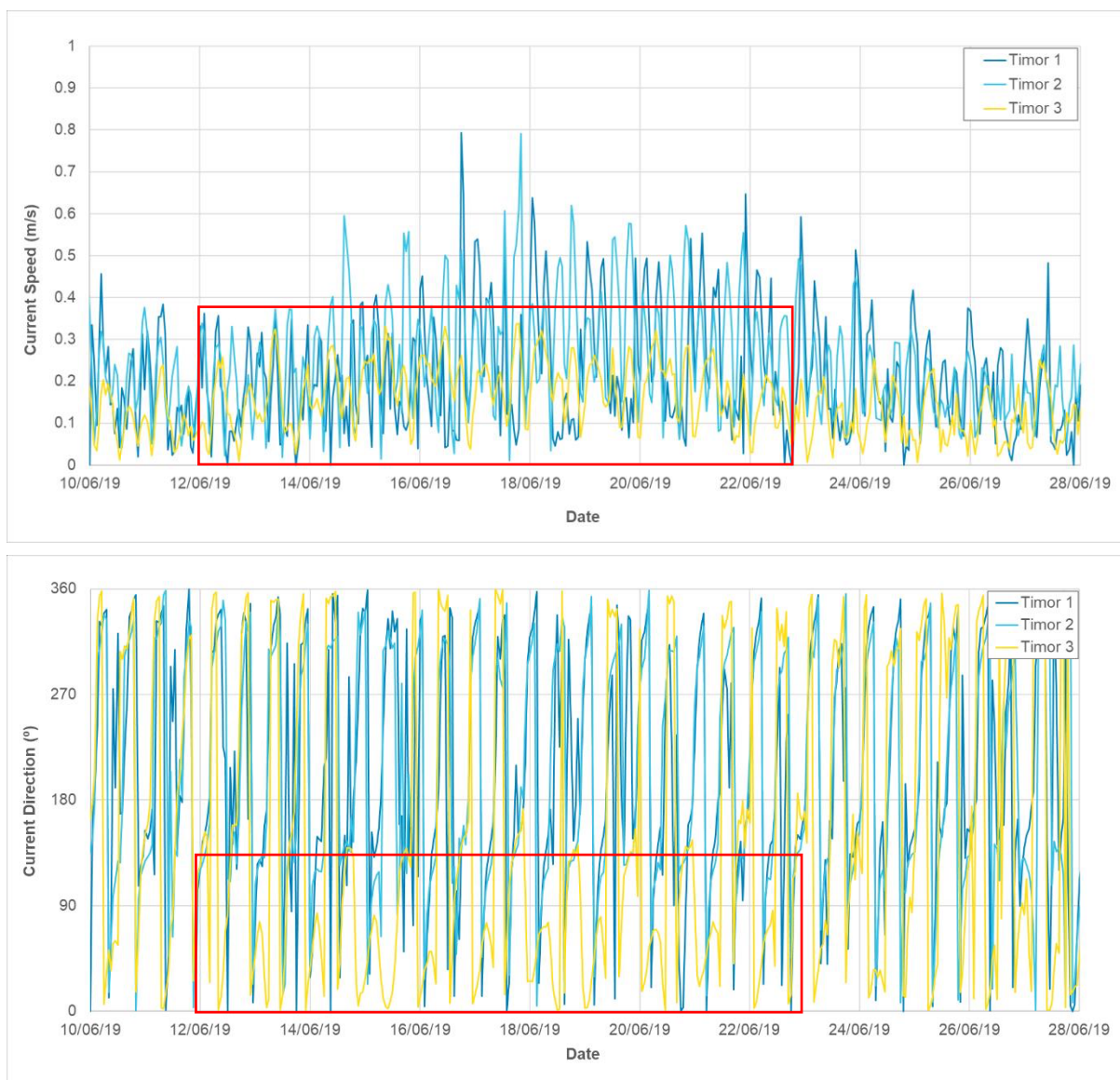
Figure 16. Measured current speed (top) and direction (bottom) at the IMOS Timor 1 to Timor 3 sites over an 18-day period in the dry season (source: IMOS, 2023).
